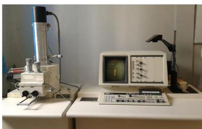
MICROSCOPE ÉLECTRONIQUE A BALAYAGE
